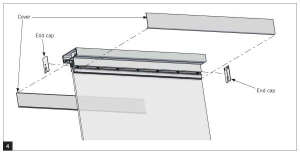
**4.1** Snap covers onto top and bottoms rails using a rubber mallet.
